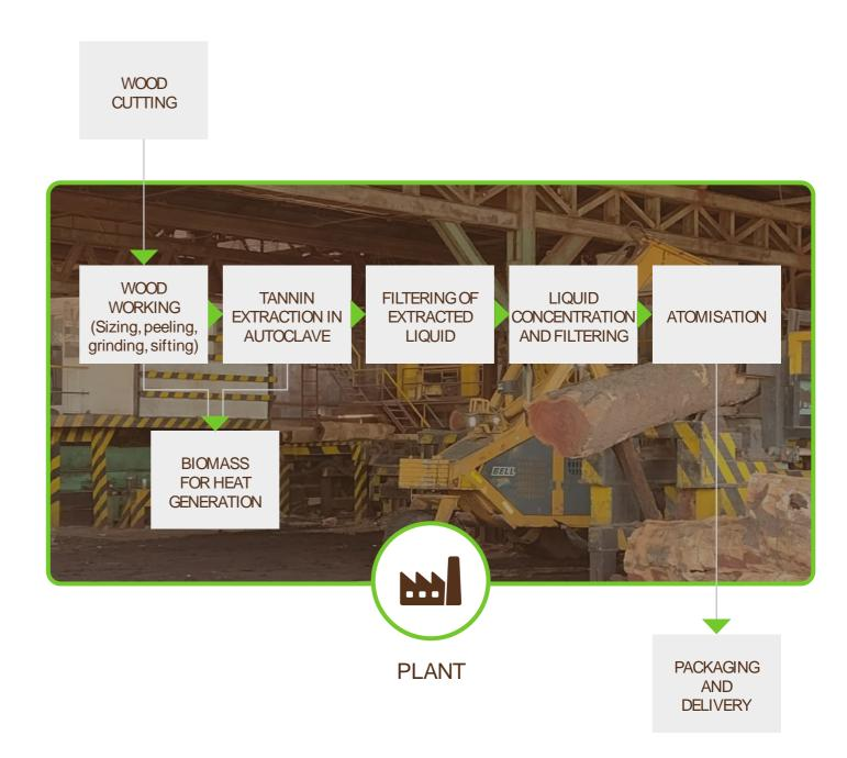
From the Silvafeed Q production a co-product is obtained, that is the exhausted wood from the tannin extraction phase, which together with other wood scraps is used to feed the co-generator owned by the Indunor plant.
